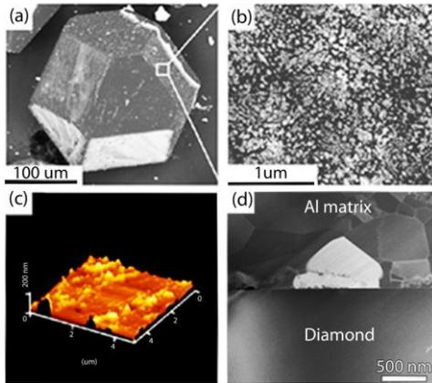
Figure 1. SEM images showing the morphologies of (a) a W-coated diamond particle, (b) deposited nanoparticles, (c) deposition thickness measured by SPM and (d) STEM/ADF image of a diamond/Al interfacial area
