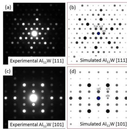
Figure 4. PED analysis of the deposited particle arrowed in Fig. 2a: (a) and (c) experimental zone-axis patterns, (b) and (d) corresponding simulated patterns of the  $Al_{12}W$  phase
