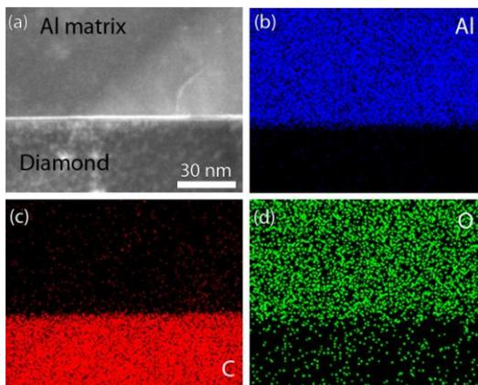
Figure 3. STEM/EDX analysis of the 'clean' diamond/Al interface: (a) ADF image, (b) corresponding Al, (c) C and (d) O elemental mappings
