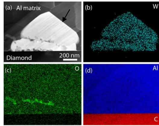
Figure 2. STEM/EDX analysis of the diamond/Al interfacial area containing a deposited particle: (a) ADF image, (b) corresponding W, (c) O and (d) mixed Al and C elemental mappings
