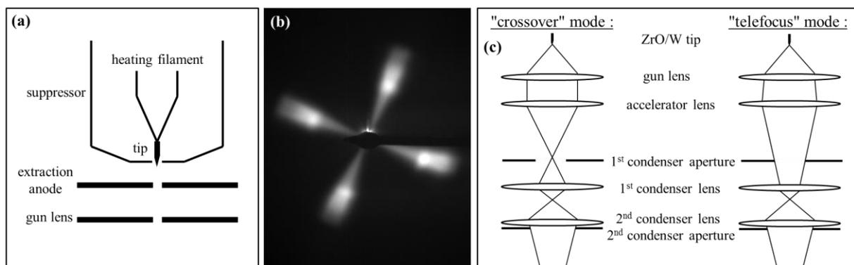
Figure 1. (a) Diagram of a SFEG, (b) image of an emission pattern of a ZrO/W tip showing side-emission lobes and a masked intense central emission from (100) facet and (c) optics diagrams of the condenser part for the two SFEG modes.
