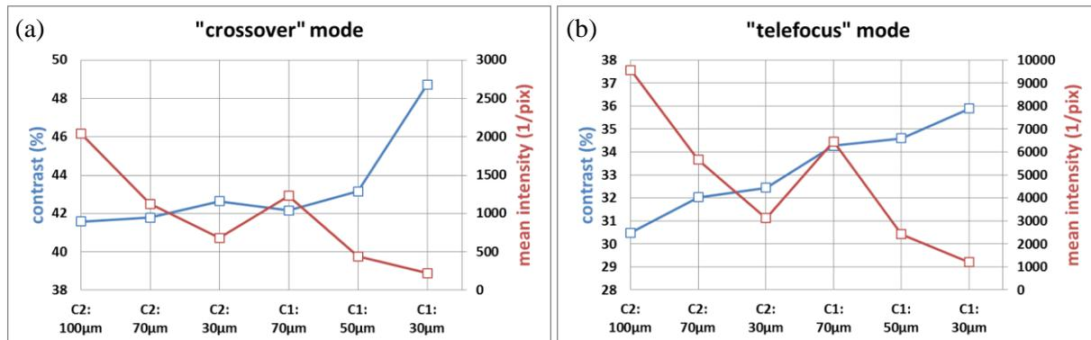
Figure 2. Hologram contrast and mean intensity in both (a) "crossover" and (b) "telefocus" modes, depending on condenser aperture conditions.
