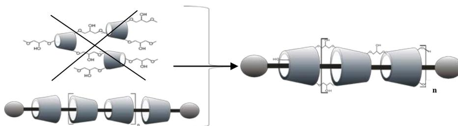
Figure 1 : Schematic synthetic route leading to the CD nanotubes
