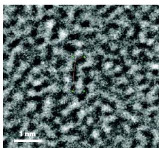
Figure 3. HRTEM images of silylated CD nanotubes obtained from 1000  $\text{g}\cdot\text{mol}^{-1}$  PEO
