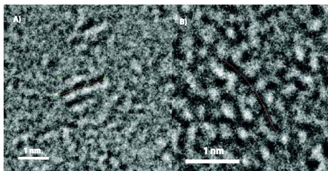
Figure 2 : HRTEM images of CD nanotubes obtained from A) 1000  $\text{g}\cdot\text{mol}^{-1}$  PEO and B) 1500  $\text{g}\cdot\text{mol}^{-1}$  PEO
