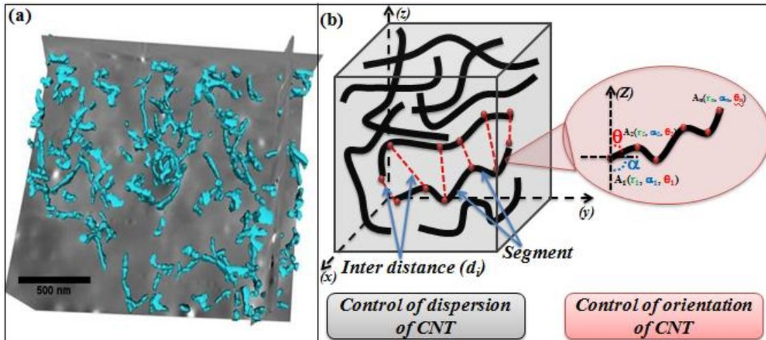
Figure 1. Control of dispersion of CNT: (a) Three dimensional model of the reconstructed volumes were in blue are showed the grafted CNT. (b) quantification of the CNT dispersion and orientation states by segmenting the CNTs into straight lines.
