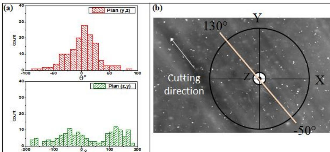
Figure 2. Control of orientation of CNT: (a) Polar angle  $\theta$  represents the orientation of each segment in the YZ plane and the azimuthal angle  $\alpha$  is the orientation of each segment in the XY plane. (b) Orientation and casting direction of CNT in the grafted samples.
