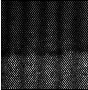
Figure 1. HAADF observation of an epitaxial Si layer (dark) on \text{Si}_{0.8}\text{Ge}_{0.2} substrate (bright). Atomic column intensity variations are due to chemical composition variations.
