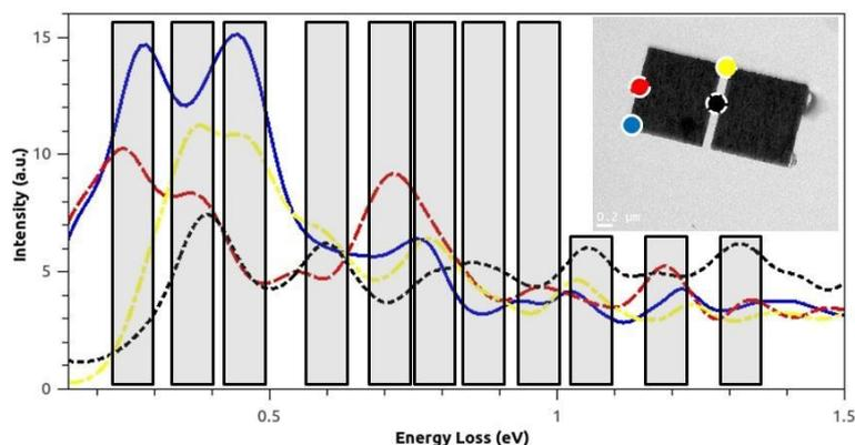
Figure 2. Spectra showing the multiple hybrid plasmon resonances peaks of the two silver squares. The spectra were extracted from four positions color coded in the inset.
