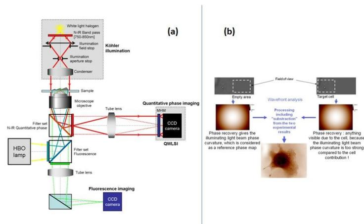
Figure 1. (a) Experimental setup. (b) General principle of the technique. A first reference wavefront is recorded without any cell in the field of view. Then a second one is recorded, with the target cell imaged on the CCD plane of the system. Both recorded wavefronts seem identical, but specific post-processing based on subtraction between them gives a highly contrasted phase image of the cell. Such a process also allows eliminating most of the phase distortion due to the optical system.
