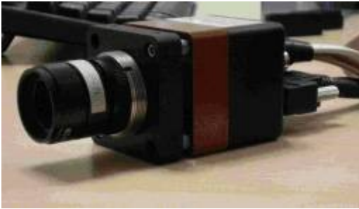
Fig.1 : solar blind camera based on AlGaN heterostructures (commercial package Raptor).
