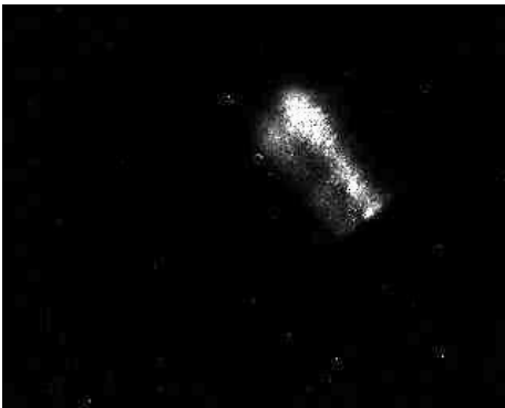
Fig.2: Image of the split beam of Soleil DISCO line taken at 130 nm by the EUV camera based on AlGaN heterostructures
