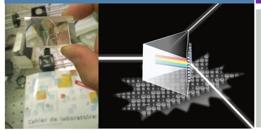
Metasurfaces can successfully mitigate the dispersion of refractive optical components leading to new achromatic applications in the visible wavelength.
