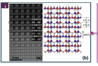
Fig 1: (a) High resolution high angle annular dark field image of a  $AI_{5+\alpha}Si_{5+\delta}N_{12}$  layer epitaxied on AIN. The insert shows a simulated image using the model presented in (b).
