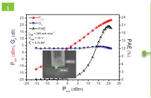
**Fig 1:** Output power, power gain and power added efficiency versus absorbed power at 40 GHz for a 2 × 50 × 0.07 µm<sup>2</sup> AlGaN/GaN HEMT on Free-Standing GaN substrate. The insert shows the 0.07 µm footprint gate.
