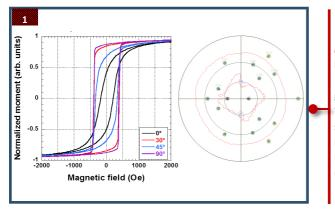
Fig 1: in-plane magnetization loops (rt) and XRD pole figure of a 150 nm-thick Fe<sub>3</sub>O<sub>4</sub> epilayer grown on m-plane nonpolar ZnO. The pole figure taken at  $2\Theta = 57^{\circ}$ shows the (5,1,1) and (3,3,3) reflections of only one single Fe<sub>3</sub>O<sub>4</sub> domain oriented along the (1-12) direction.
