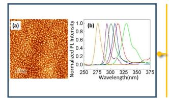
Fig (a) : Atomic force microscopy image of AlGaN quantum dots grown by molecular beam epitaxy.
