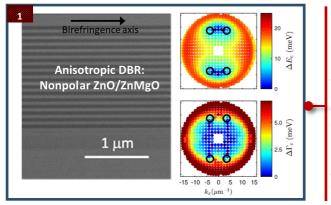
Fig 1: Cross-section SEM image of an anisotropic optical microcavity based on nonpolar ZnO/ ZnMqO DBR (left) displaying Voigt Exceptional points. Energy difference (top right) and FWHM difference (bottom right) between the two eigenmodes of the cavity as a function of inplane momentum. The four exceptional points are indicated by
