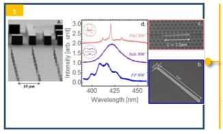
**Fig 1** : SEM images of (a) bird's eye view of a NW array obtained after selective-area sublimation. (b) A NW transferred on SiN. (c) A subwavelength NW embedded in a slotted photonic crystal. (d) Room-temperature μPL spectra of the NW shown in panel b (blue line), a subwavelength NW transferred on SiN (purple line) and the subwavelength NW embedded in a photonic crystal shown in panel c (pink line)
