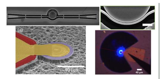
Top: A III-nitride photonic circuit combining a microdisk resonator with bus waveguides for light collection and outcoupling gratings. The distance between the microdisk and the bus waveguide is in the tens of nm range.
