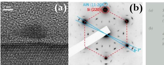
Side view of an AIN island deposited on Si (111).
