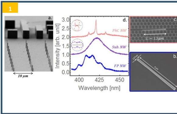
**Fig 1 :** SEM images of (a) bird's eye view of a NW array obtained after selective-area sublimation. (b) A NW transferred on SiN. (c) A subwavelength NW embedded in a slotted photonic crystal. (d) Room-temperature  $\mu$ PL spectra of the NW shown in panel b (blue line), a subwavelength NW transferred on SiN (purple line) and the subwavelength NW embedded in a photonic crystal shown in panel c (pink line)
