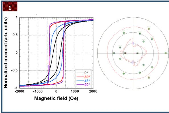
**Fig 1:** in-plane magnetization loops (rt) and XRD pole figure of a 150 nm-thick  $\text{Fe}_3\text{O}_4$  epilayer grown on m-plane nonpolar ZnO. The pole figure taken at  $2\theta = 57^\circ$  shows the (5,1,1) and (3,3,3) reflections of only one single  $\text{Fe}_3\text{O}_4$  domain oriented along the (1-12) direction.
