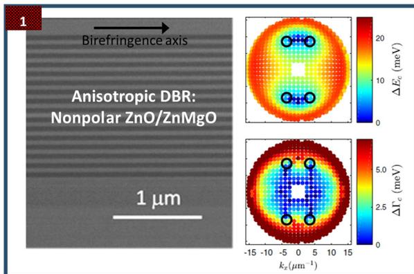
**Fig 1:** Cross-section SEM image of an anisotropic optical microcavity based on nonpolar ZnO/ZnMgO DBR (left) displaying Voigt Exceptional points. Energy difference (top right) and FWHM difference (bottom right) between the two eigenmodes of the cavity as a function of in-plane momentum. The four exceptional points are indicated by
