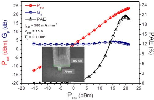
**Fig 1:** Output power, power gain and power added efficiency versus absorbed power at 40 GHz for a  $2 \times 50 \times 0.07 \mu\text{m}^2$  AlGaIn/GaN HEMT on Free-Standing GaN substrate. The insert shows the  $0.07 \mu\text{m}$  footprint gate.
