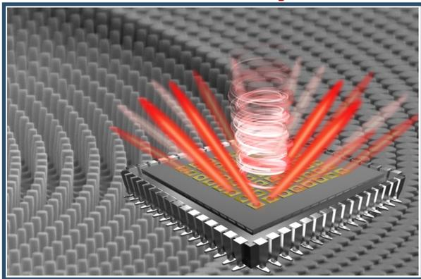
*Programmable lasers array for wide-range dynamic beam steering. The image shows a schematic of the metasurface integrated vertical surface emitting array (MS-VCSELS). The array of MS-VCSELS is mounted onto a PCB board, indicating different deflection angles for wide-range dynamic beam steering applications. Below, a SEM of the nanopillars forming the beam shaping metasurfaces.*
